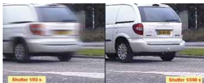
Bosch Dinion XF Motion Blur Reduction. Shutter control increases shutter speed from 1/50 sec to 1/500 sec as light decreases
